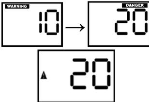
For ToxiPro instruments with a toxic sensor and with the STEL and TWA alarms enabled, the ToxiPro will briefly show the STEL and TWA alarm levels.
